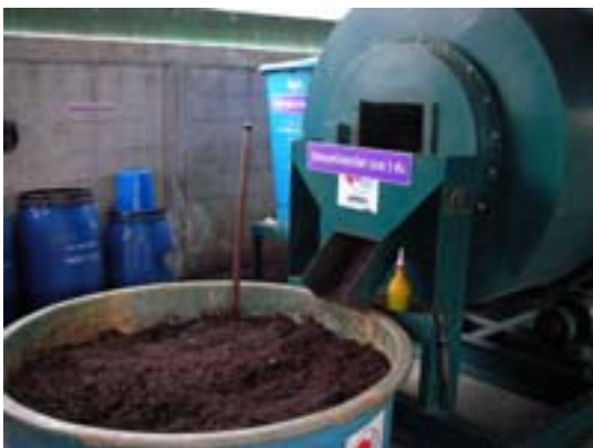
Rotary bin to remove excess moisture.
